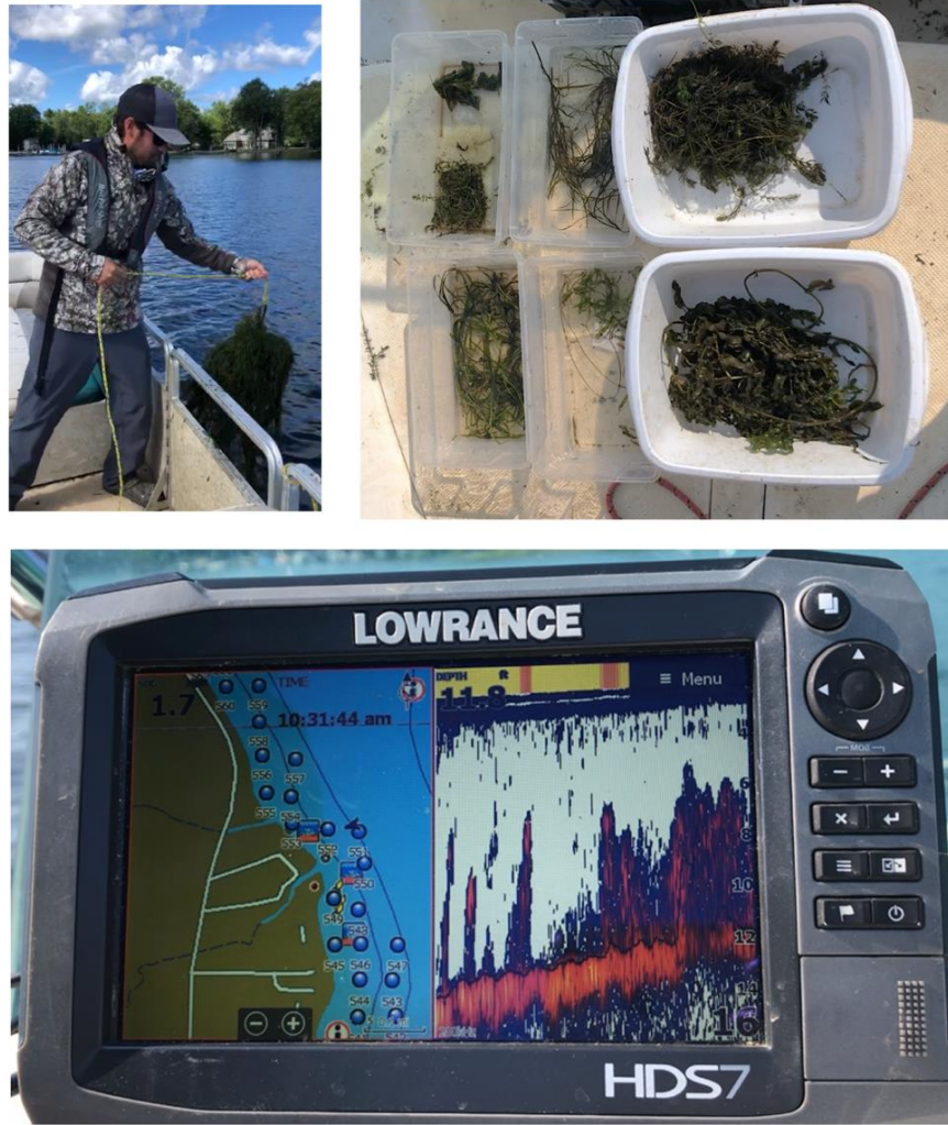
Figure 1: Retrieving and sorting SAV by species (Top) while concurrently recording sonar/SAV biovolume data throughout the littoral zone of Chautauqua Lake (Bottom).
